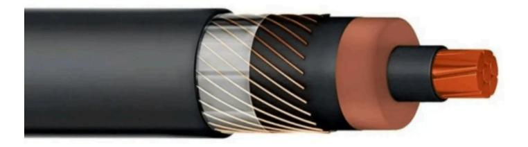
1-) Conductor: Bare electrolytic copper wires, soft temper, class 2 or 5 stringing, according to NBR NM 280; 2-) **Conductor Shielding:**
