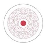
CONDUCTOR: Formed by electrolytic bare copper wires or tinned, soft temper, class 5 stranding.
