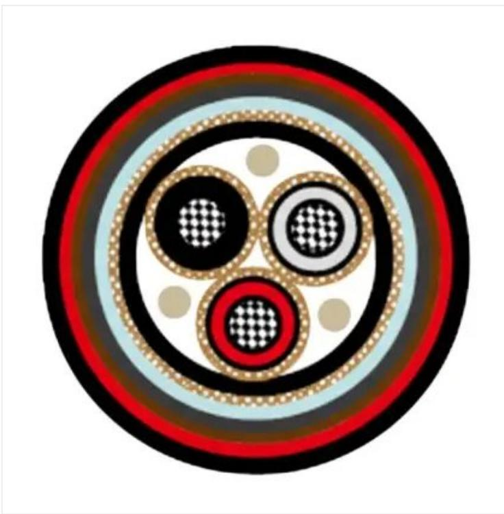
HydroCore® Cabo Naval NEK 606 Water Blocked P30 RFOU-HCF / TFOU-HCF; 6/10(12) kV;
